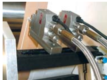
Length pasting by nozzle application
