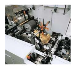
Adjustment of first and second gripper of bottom folding drum is made centrally or individually for each side and is possible even while the machine is in operation (option). All bottom stations are adjusted at the same time through a gear segment.
