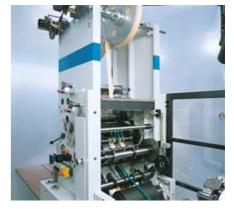
Different bottom cover sheet units feature up to 100 % coverage of paste. The station is optionally available with a flexo printing unit or a register control.
