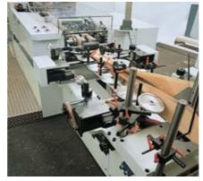
The gusset depth at the tube forming station is set via servo motors (option). Fine corrections can be made during production, from the central control panel. All data can be stored and recalled.
