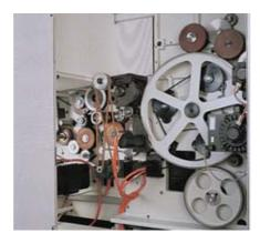
The cut-off station is equipped with a rotating knife, which can be set up with either straight cut or serrated cut.
