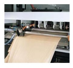
Fine adjustment of the servo driven (option) cutting tools is done manually. The length glueing nozzles are engaged and closed pneumatically.
