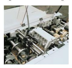
Fine adjustments by servo drives (option) via operator control panel.
