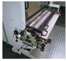
The lining device is driven by servo motors (option) and is equipped with a fast lift-off system and idle drive.
