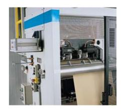
Integrated into the infeed station is a servo driven (option) incision device for different cutting tools for special bags such as vacuum cleaner bags.
